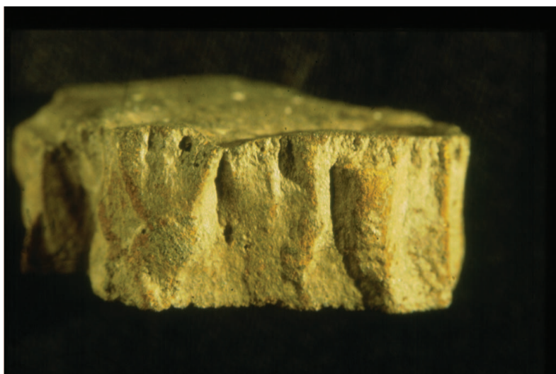
Figure 10. Side view of a slag fragment from Saint-Véran showing the typical prismatic layer 1–2 mm below the upper surface (total thickness ~10 mm)
